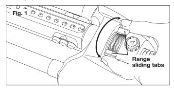
For full coverage, spread the tabs apart (Fig. 2). For a narrower range, bring the tabs closer together (Fig. 3). Bring both tabs fully to either the left (Fig. 4) or the right (Fig. 5) for coverage on either side.
